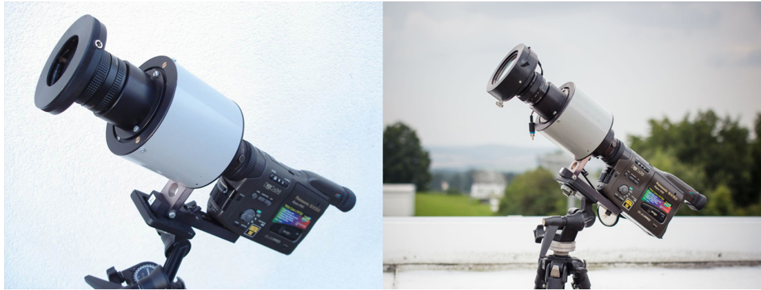
Figure 3.1: Pictures of used equipment. Direct camera with Mullard image intensifier on the left, spectral camera setup on the right.
