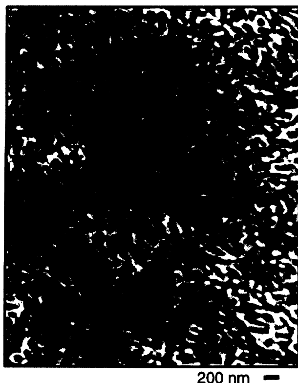
Figure 7: TEM photo of bicontinuous microemulsion morphology; ternary system of polyethylene / poly(ethylene-propylene) / polyethylene- b -poly(ethylene-propylene); 10 % of diblock copolymer. Adopted from [36].
