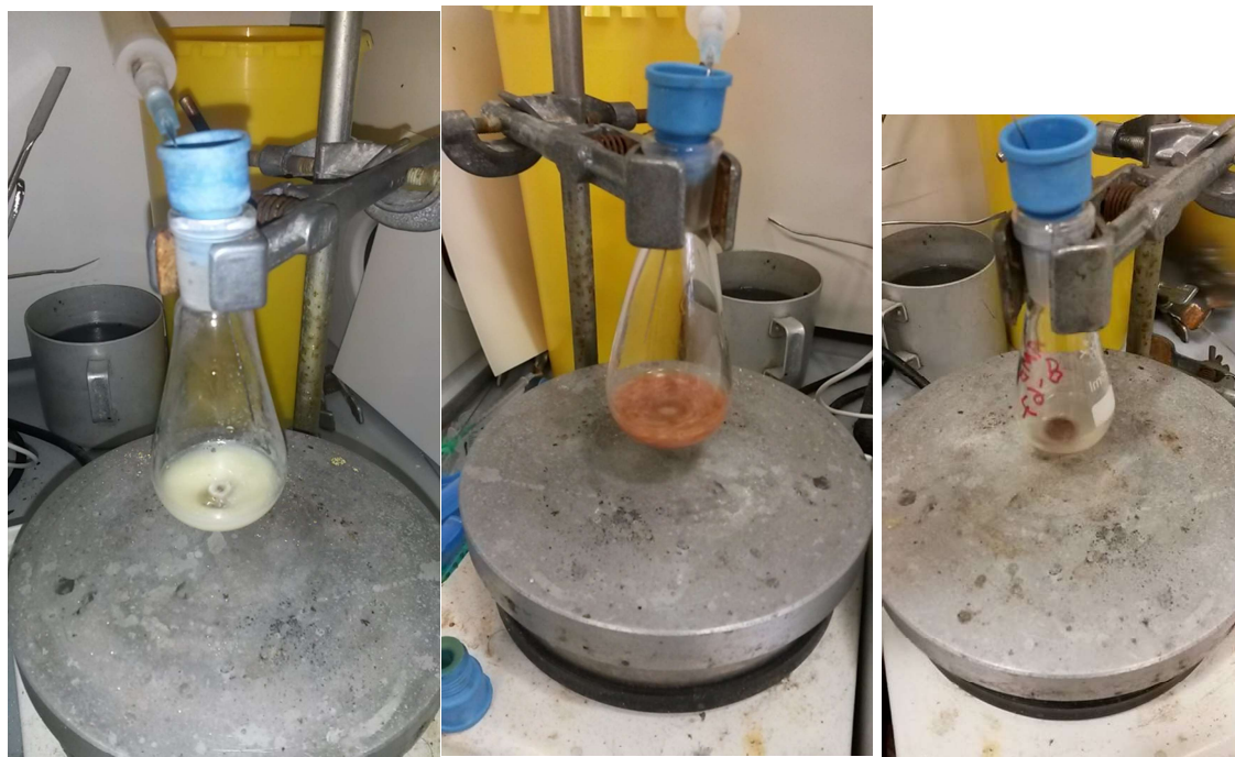
Figure 3.18: Pictures taken after formation of the anhydroses. Left: Completed conversion of 3.20 to anhydrose 3.28 . Middle: Completed conversion of 3.21 to anhydrose 3.30 . Right: Completed conversion of 3.22 to anhydrose 3.32 . All three pictures were taken after stirring at room temperature for 15 minutes.
