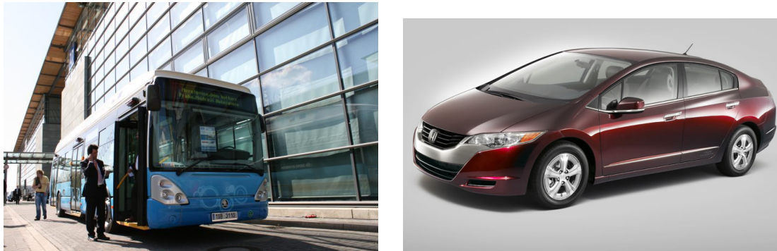
Fig. 2.1: Examples of use of trihybride: fuel cell/energy storage element/super capacitor. On the left is example of the trihybrid bus which is constructed by Škoda Electric Pilsen trolley bus and Fuel cell manufacturer is Proton Motors [40]. On the right is a sport car Honda Clarity with PEM FC solution of 80 kW [41].
