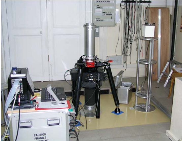
Fig. 4.2. Absolute gravimeter FG-5 and relative gravimeter LaCoste&Romberg D-188 (IG ASCR, Prague) during the world comparison and calibration campaign of absolute and relative gravimeters in Sevres, Paris. Author participated in two of those campaigns in 2001 and 2005 (e.g. Vitushkin et al., 2002) with the aim, beside others, to investigate the stability of the calibration function. Standard deviation of LCR-D188 was about 2 \mu Gal. Here LCR-D (right up) is measuring vertical gradients nearby FG-5 location. (Photo J.Mrlina)
