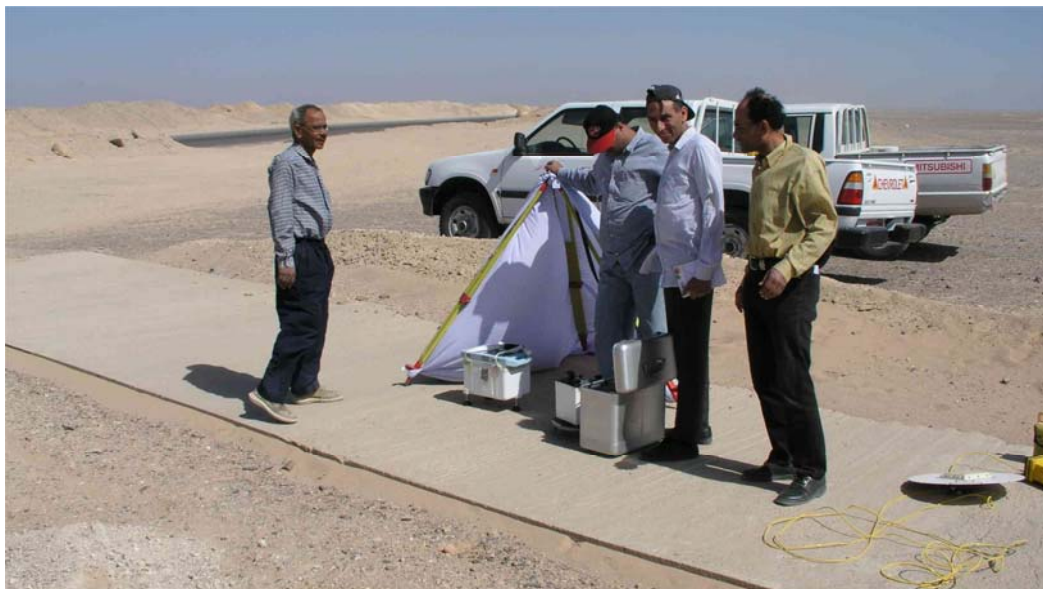
Fig. 4.3. My colleagues were trying to keep protection, but even on a huge concrete platform we felt the strong wind effect on gravity readings (geodynamic investigations in Egypt). Here we used a blanket on a geodetic tripod. Later on, the wind cut the blanket to pieces.
