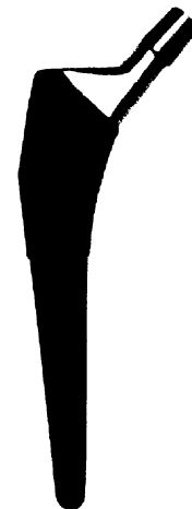
8.2 – necementovaný dřík (podle Information for Patients of Total Hip Replacement, or Total Hip Arthroplasty (THA), 2006)
