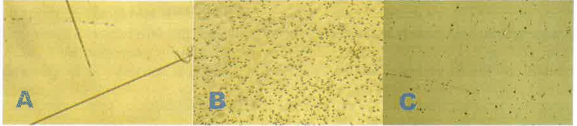
Figure 7.35: Photographs of the surface of Ce:LuAG thin films prepared from the BaO-based flux. A is the surface of the sample 1L2 - LuAG layer on LuAG substrate, Table 7.3. It has the smooth surface. The lines comes from scratches in the substrate originating in the polishing procedure. B is the surface of the sample 1LC1 - Ce:LuAG layer on LuAG substrate. The surface is not uniform, with a lot of defects and scatters the light strongly. C is the surface of the sample 1LC2 - Ce:LuAG layer on LuAG substrate. The surface has much better quality than in the case of the sample 1LC1. There are only a few defects.
