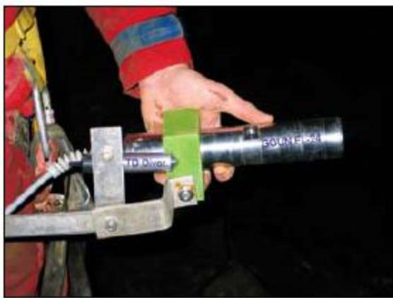
Obr. 11: Fluorometr GGUN-FL24 (Gabrovšek a kol., 2010)
