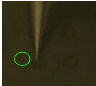
Figure 6.25: A picture of an electrode contacted by a BeCu probe tip after application of +3 V for 30 minutes.
