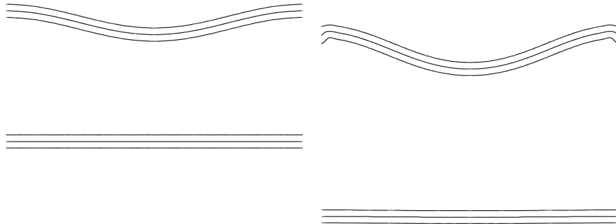
Figure 5.12: Evolution of OE and MO interfaces for single pore experiment. Initial configuration is shown on the left ( t = 0 s). On the right interfaces after 335 s are portrayed. Contours (0.1, 0.5 and 0.9) of level-set functions are included.
