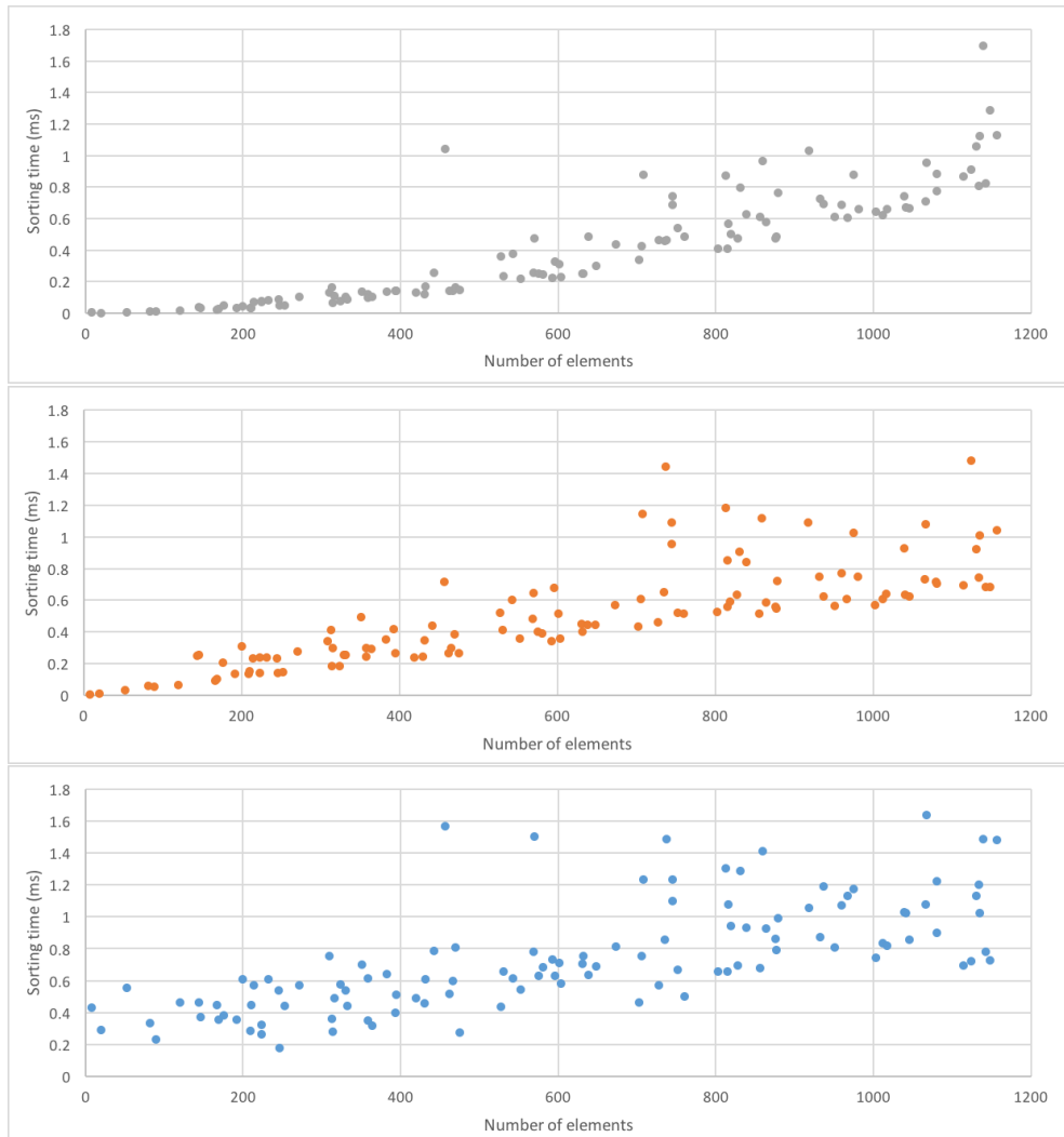
Figure 6.2: Detailed view of the sorting times of sequences of different sizes using selection sort, quick sort and a combined function (from top to bottom).
