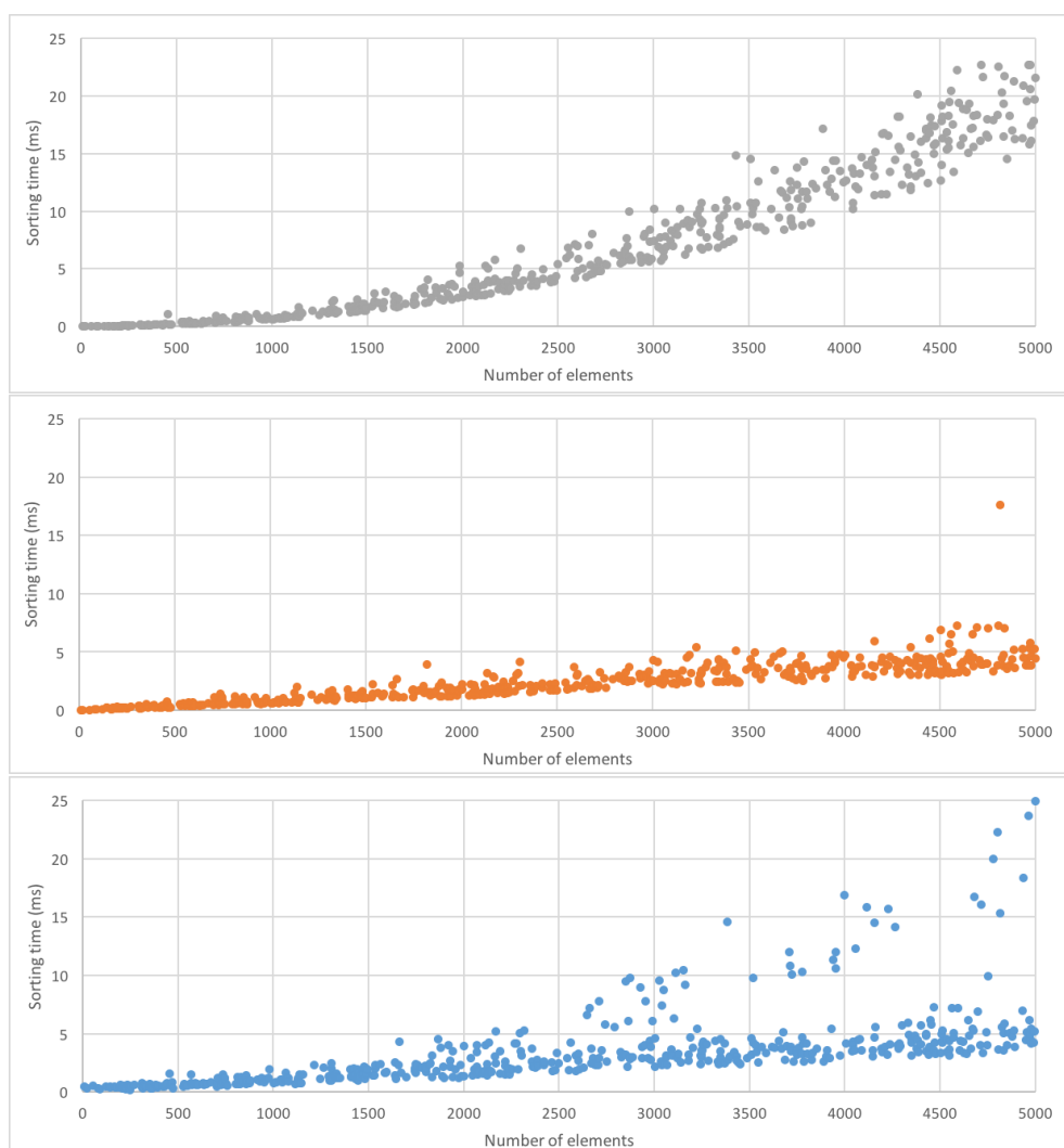
Figure 6.1: Sorting times of sequences of different sizes using selection sort, quick sort and a combined function (from top to bottom).
