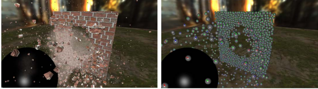
Figure 1.8: View of final rendering with generated dust and debris (left) and equivalent view showing underlying EDEM elements (right). Source: Imagire et al. [10]
