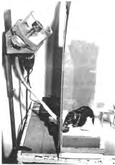
Fig.1: The apparatus used in Experiment 1 (Nekovarova and Klement, 2006). The apparatus consisted of a Skinner box with a lever and a feeder, and of a computer screen placed in front of the box. Correct operant responses were rewarded by delivery of pellets to the feeder.
