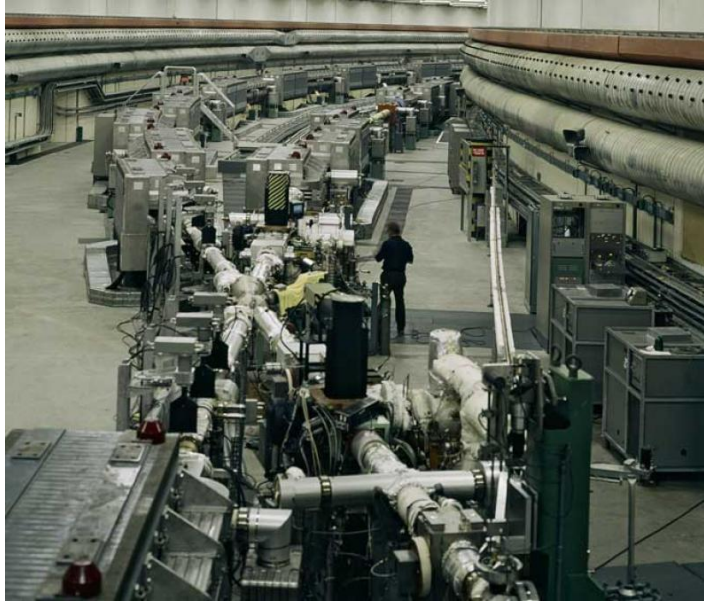
Figure 1: The world's first proton-proton collider - ISR. Two beam pipes cross at large crossing angle (Image: CERN).
