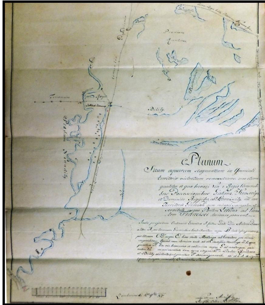
Figure 4. Plan made by Petar Aradski for the drainage of the redundant water from the territories of Gakovo, Kruševlje, Riđica, and Stanišić (1827), through the river Mostonga and consequently to the Emperor Francis Canal (bottom left corner), with the depiction of the flooded areas of Bilić and Rančevo (top right). Source: Historical Archive of Sombor Acta Politica 1358/827.
