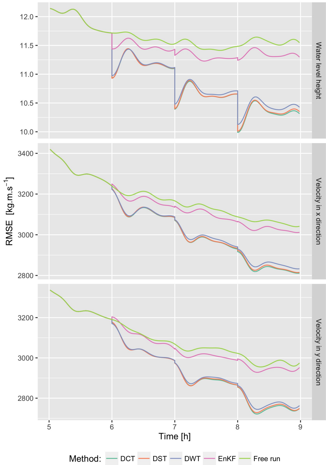
Figure 8.7: RMSE from one realization of three assimilation cycles using shallow water equations. The size of the ensemble is 20, and the observations are available every hour from 6 h until 8 h. Only the water level height is observed.
