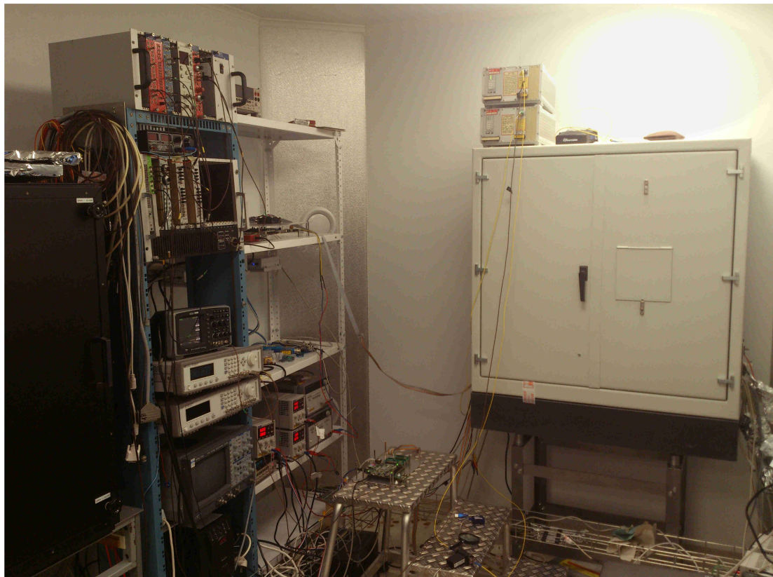
Figure 3.5: A photograph of the clean room where all tests were performed. The big white box on the right side of the picture is a black box. The two smaller boxes on it are the red and infrared lasers. Finally on the left side of the picture there are power supplies and pulse generator.
