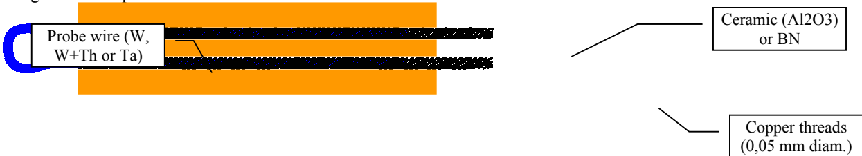
FIGURE 1. Schematic of the probe construction. Inside the ceramic the probe wire is spliced with thin copper wires. The connection between the two materials is very tight and provides an excellent mechanical and electrical contact. The covering of the probe wire with copper threads is denser than shown here for clarity.
