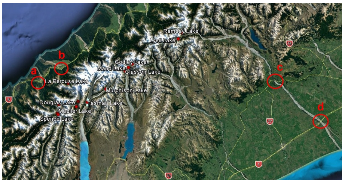
Figure 57: Map showing the intersection of potential flood paths with main roads of the South Island. (a) shows the location of SH-6 crossing the Karangarua river, (b) the crossing of SH-6 with the Cook river, (c) the crossing of the Rakaia river with SH-71, and (d) the crossing of the Rakaia river with SH-1. Source of the satellite image: Google Earth.
