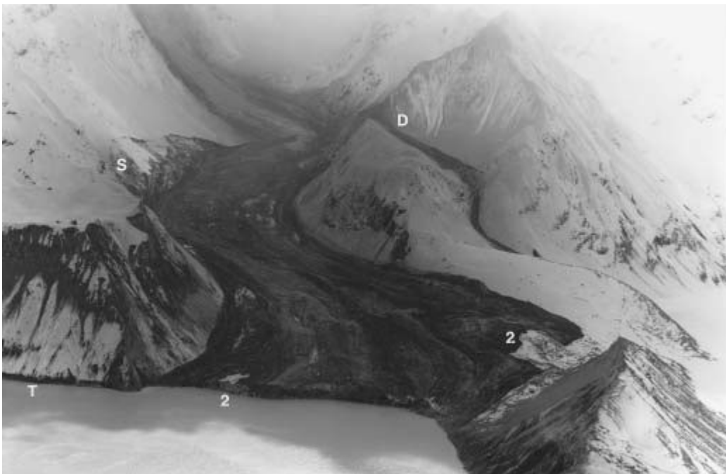
Figure 38. Sinuous path of Mount Fletcher rock avalanche of September 16, 1992. Note thin stream of debris in side valley (D), and superelevation of landslide debris (S) at bend in avalanche flow path on Maud Glacier. Points at 2 are snow-covered remnants of rock-avalanche deposit of May 2. Black trimline (T) to 7 m above lake is from wave generated by avalanche that displaced \sim 5 \times 10^6 \text{ m}^3 of water from lake. Source: McSaveney 2002.
