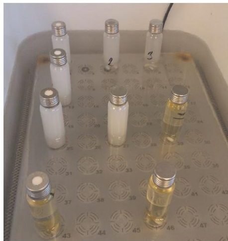
Fig. 6. Visible differences in the macroscopic appearance of the tested diosmin samples in the buffer medium pH 7.8; vials with the content of diosmin dissolved from nanofibrous membrane are transparent – yellowish (in the front and right side), versus vials with only suspended (undissolved) white diosmin particles of both the powders tested.
