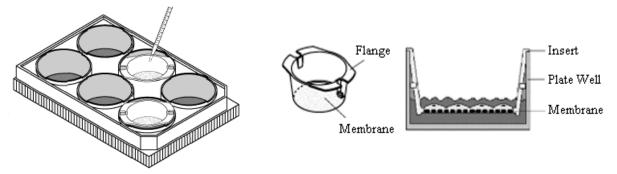
Fig. 3.2: Transwell model The 6-well plate with six chambers and inserts, detail of an insert and a side view. Source: Beckton and Dickinson, 2009.
