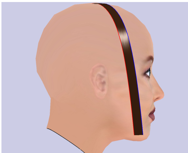
Figure 3.14: Flat wisp represented as a quad strip. Rim strands highlighted in colour.
