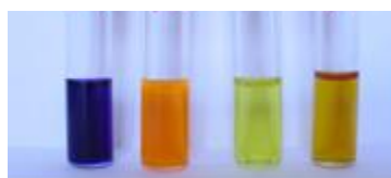
Figure 71. The DMSO solutions of compounds 53 , 54 , 52 , 56 (from left to right) several hours after preparation. The solutions were colorless immediately after dissolution.
