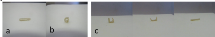
Fig. 8 SM effect of the epoxy-silica nanocomposite: a) original shape, b) heated, bended and cooled sample, c) reheating up to T_d - 10s, 20s, 30s.
