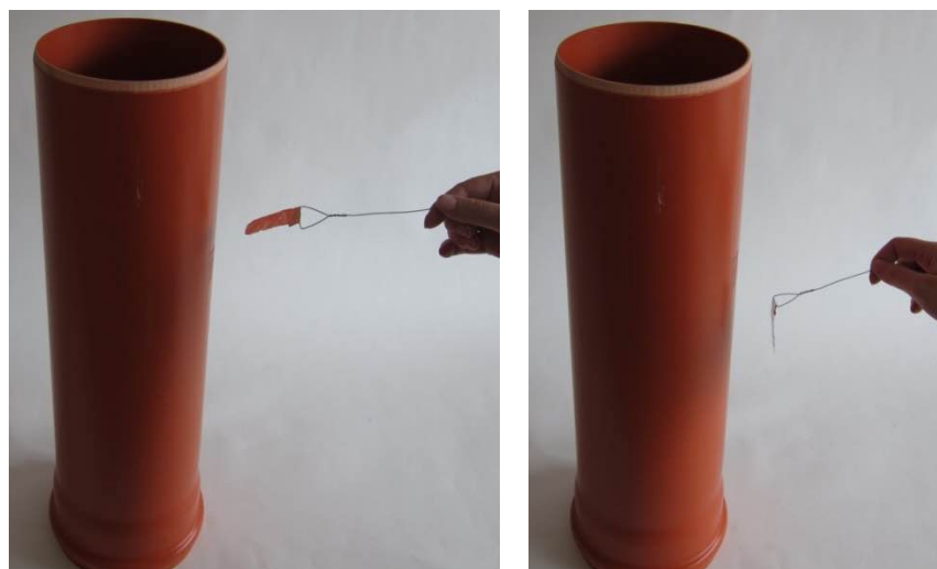
Figure 2. Arrangement of the experiment – charged place on sewage pipe (left) and place without charge (right)
