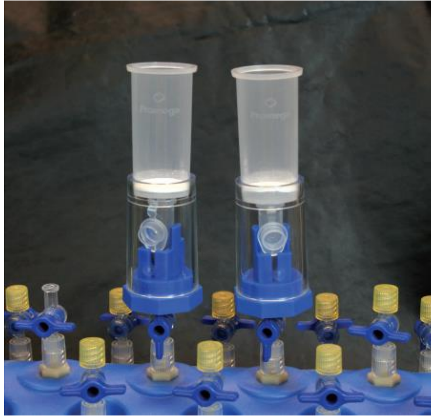
Fig. 14: Right position of the epp. tubes on the base of the Eluator™ Vacuum Elution Device
