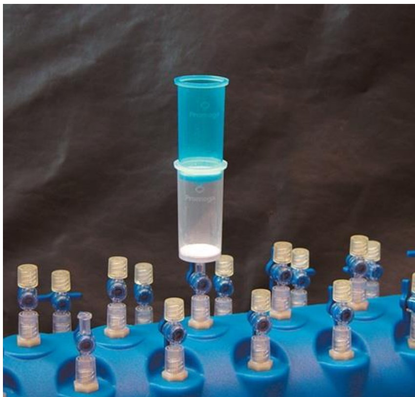
Fig. 13: Column positions on the vacuum manifold
