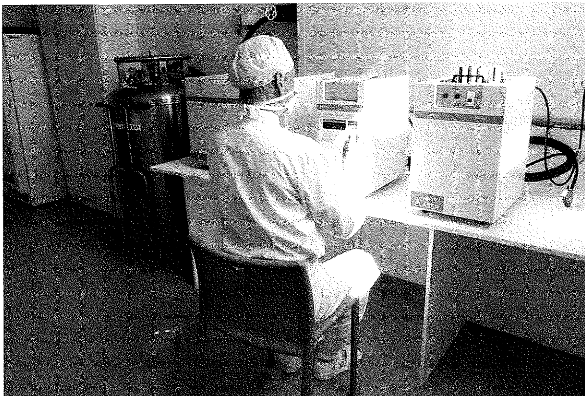
Figure 4: The programmable freezer is supplied with the liquid nitrogen from a low-pressure, 230 l container. The back-up vessel is connected to the external vessel by the tubing.
