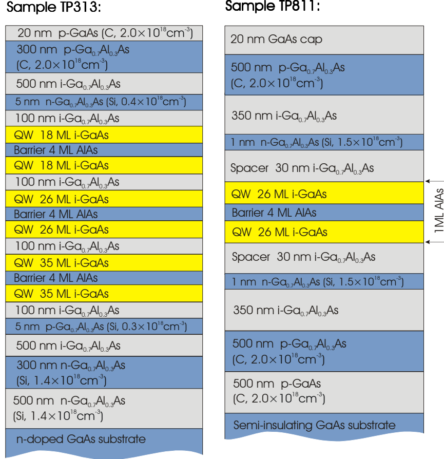
Figure 7.3: The MBE-grown sequence of layers for samples TP313 and TP811. The widths of layers are not in scale.
