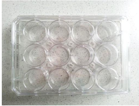
Fig. 14. A modified 12-well plate with holes in the bottom.
