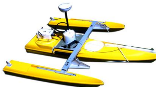
Obr. 2.5: SonTek hydroboard (SonTek, 2010)
