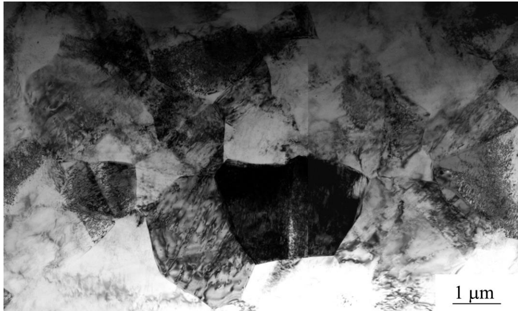
Figure 5.5: Transmission electron micrograph of extruded AZ31 alloy.
