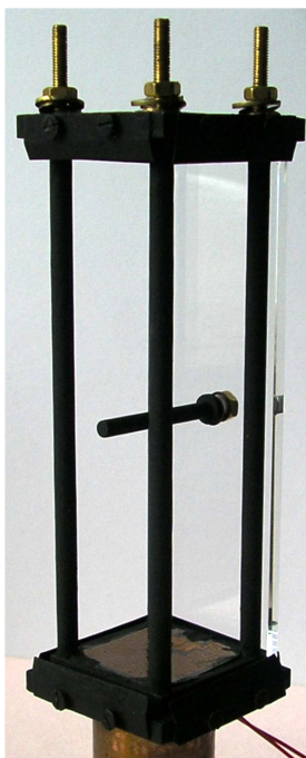
Figure 2.4 Photograph of the experimental cell. The shown cylinder was used for a series of experiments (see below) and can be removed.
