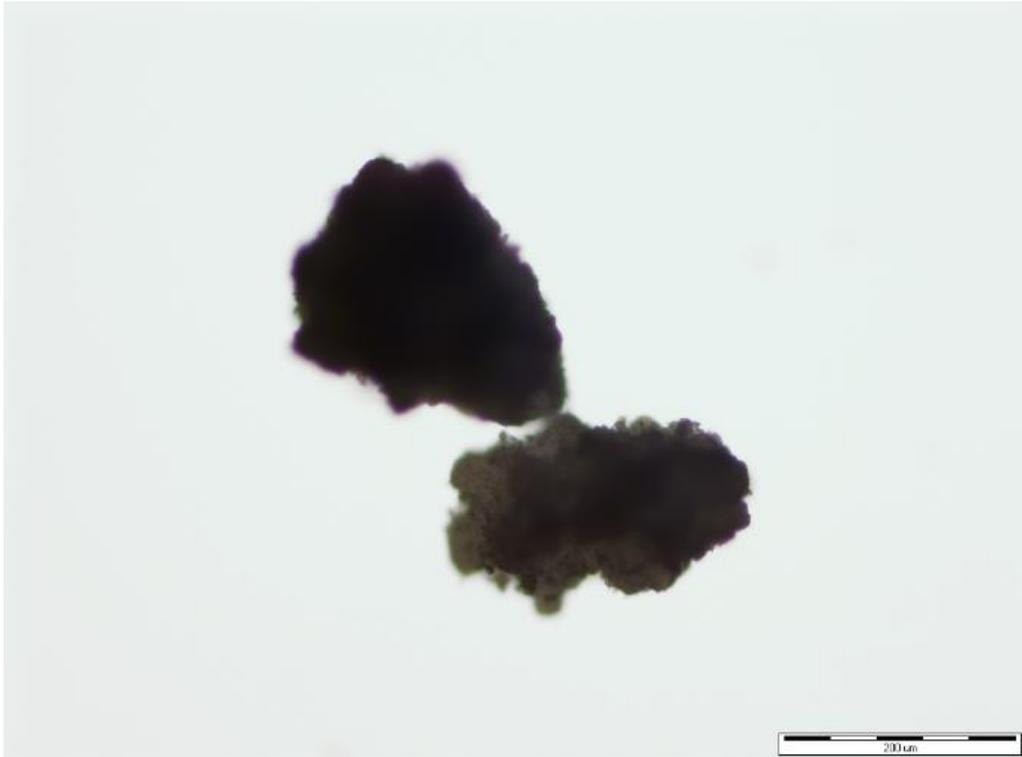
Figure 6: Picture of DI-CAFOS A150 obtained from optical microscope (magnification 10X)
