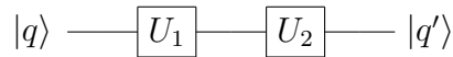
Figure 1.2: Simple single qubit quantum circuit. The time flows from left to right.
