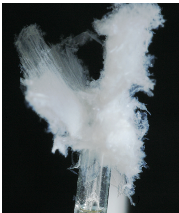
Figure 5.1: Picture of Ti-NT look like a feathers, glass capillary has diameter approximately 0.5 mm.
