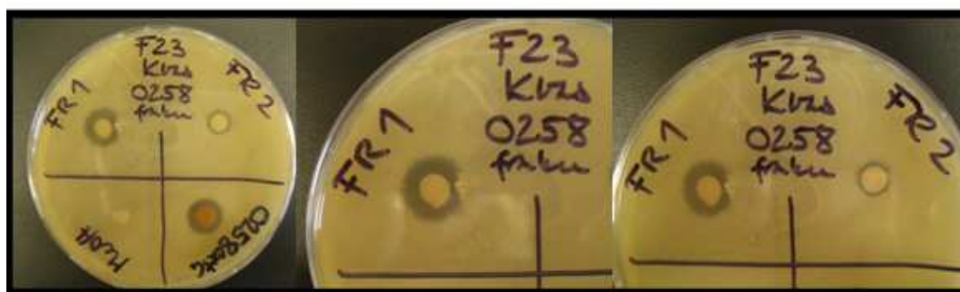
Figure 22. Antimicrobial activity testing of fraction isolated with HPLC-UV iso method using Kirby-Bauer disk diffusion susceptibility test.
