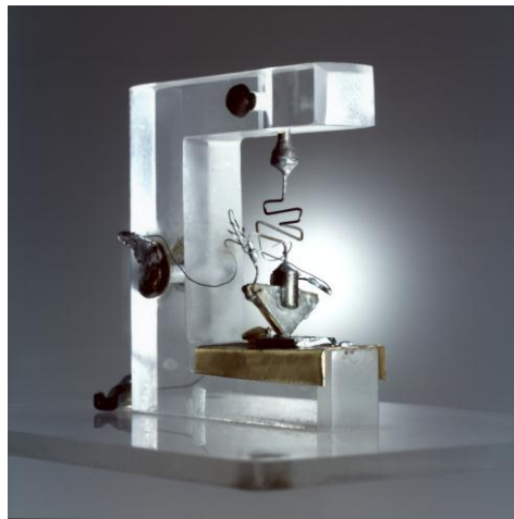
Figure 1.1 The first transistor. Image courtesy of Bell Labs.
