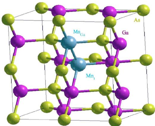
Fig. 1: (Ga,Mn)As unit cell. The most energetically favorable position of Mn atom in the GaAs host cell is in the position of Ga ( $Mn_{Ga}$ ). The less common interstitial position is depicted as  $Mn_I$ . [27]
