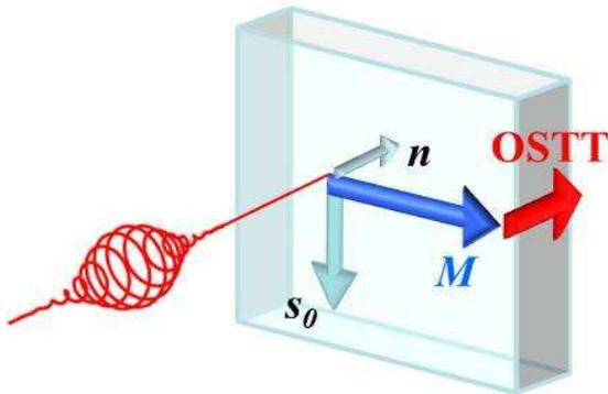
Fig. 10: Schematic illustration of the optical spin transfer torque. The circularly polarized light generates the carrier spin polarization, where the initial orientation of spins ( $\mathbf{n}$ ) is parallel with the incident light direction and perpendicular to magnetization ( $\mathbf{M}$ ). The steady-state component of the injected spin density ( $s_0$ ) is oriented in the sample plane, perpendicular to  $\mathbf{M}$ , and exerts a torque on the magnetization vector  $\mathbf{M}$ .
