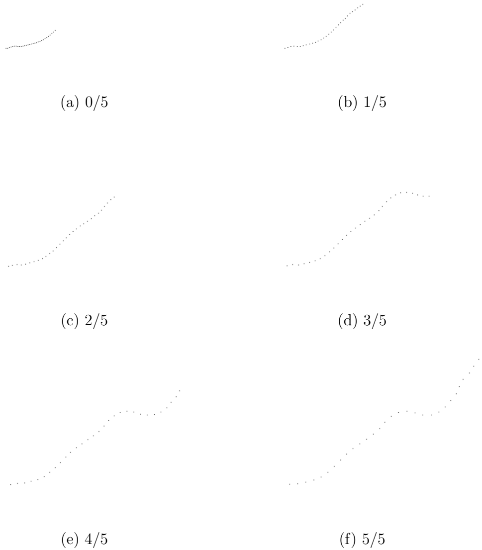
Figure 2.14: Tracking of skeleton control points within the interval between acquisitions of images in Figure 2.11; their positions were computed by shrinking of the filament of the morphological skeleton from the latter observation session (f), see Figure 2.13b, to the length of the filament from the early session (a), see Figure 2.13a.
