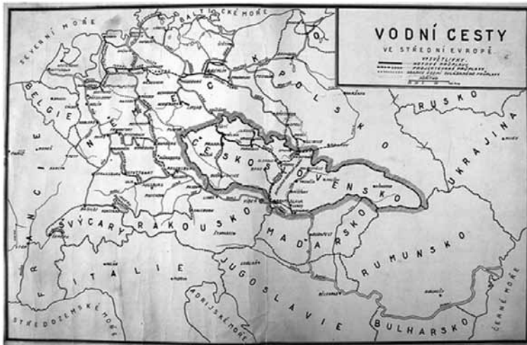
Figure 2.8 – Detail from the undated waterway map of Central Europe from the ŘVC archives, covering the full Czechoslovak waterway program: the DOE, canalization of the Vltava upstream from the Elbe and the river Váh in Slovakia. The projected national grid on the map shows how the Paris Treaty complicated infrastructural development in the region – compare with figures 2.3 and 2.4. The pencil line indicates the actual border between Poland and Germany and, together with the printed border line, delineates the Upper Silesia region that voted for loyalty to Germany in 1921. The map also shows the short-lived state border between Russia and Ukraine. Note that the author designed the map to include Paris (Paříž, in the left margin); perhaps in order to emphasize the westness of the network and its non-German character. The dotted line just below the city of Plzeň (Pilsen) in Bohemia delimits “territory controlled by the canal.” Source: Vodní cesty ve Střední Evropě (NAČR, GRVC, b. 412, undated).
