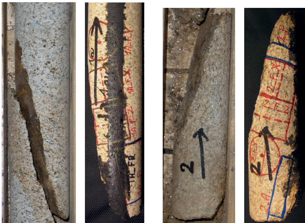
Figure A1 (continued on the following four pages). Borehole core samples shown on photographs taken prior to extraction from the core boxes (left) and after marking of position of the TC scanning profiles and of the plugs for permeability and V_p measurements (right). The core diameter 4.45 cm represents the scale. Where present, the bold black marker indicates the sample name (number) and direction towards the top of the borehole (arrow). The TC scanning profiles are represented by black painting stripes parallel to the core axis. The positions of the plugs for permeability and V_p measurements are indicated by red marker.
