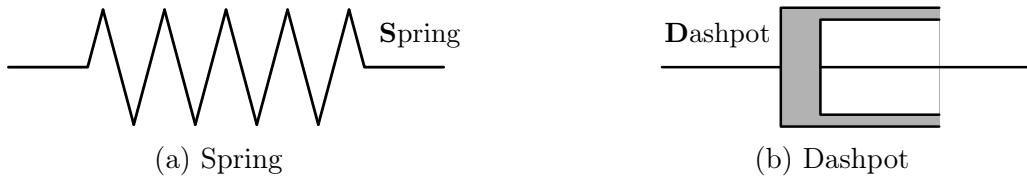
Figure 1.22: Linear spring and linear dashpot.
