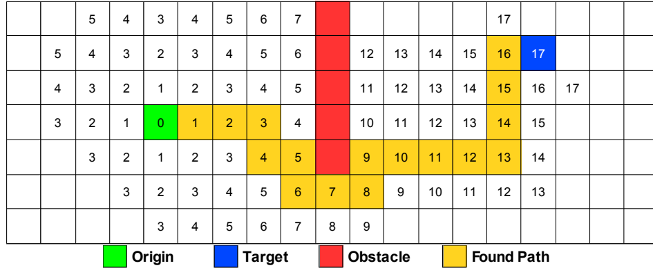
Figure 13: Pathfinding performed using the A* with Manhattan heuristic. It visited 84 tiles.
