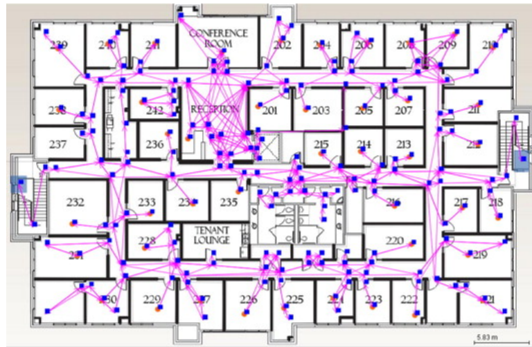
Figure 8: An example of a navigation graph for pathfinding.
