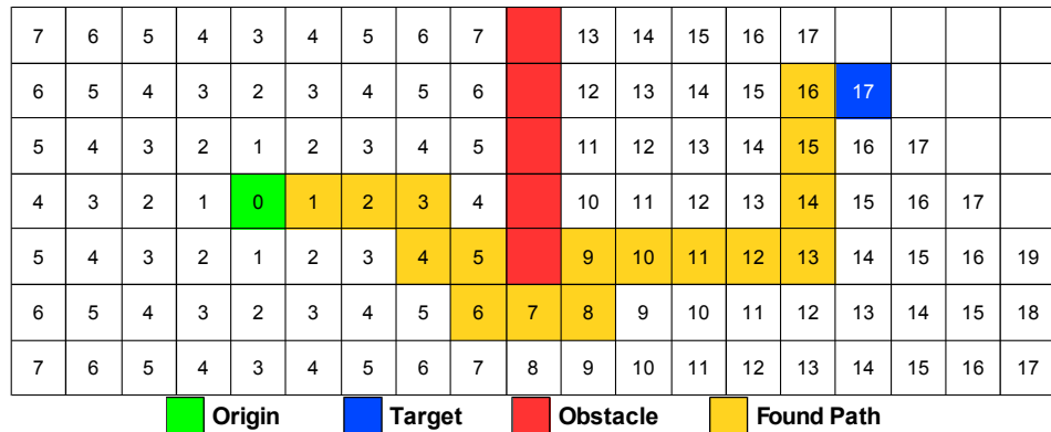
Figure 12: Pathfinding using the Dijkstra's algorithm. It visited 111 tiles.
