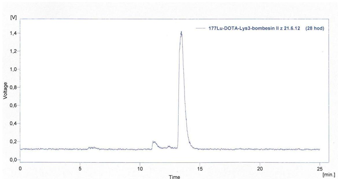
Figure 10: Quality control of  $^{177}\text{Lu}$ -DOTA-Lys3-Bombesin prepared 4 months after preservation of the cold peptide at  $-20^{\circ}\text{C}$ , labeling conditions (pH 5.02,  $42^{\circ}\text{C}$ , and heating time 40 minutes), HPLC analysis 15 minutes after radiolabeling
