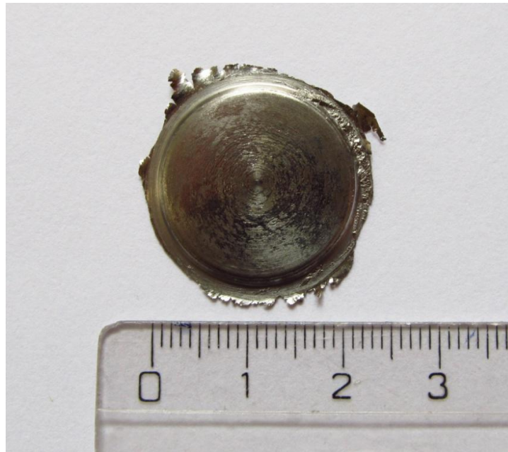
Fig. 3.3 Sample surrounded by the leaked material
