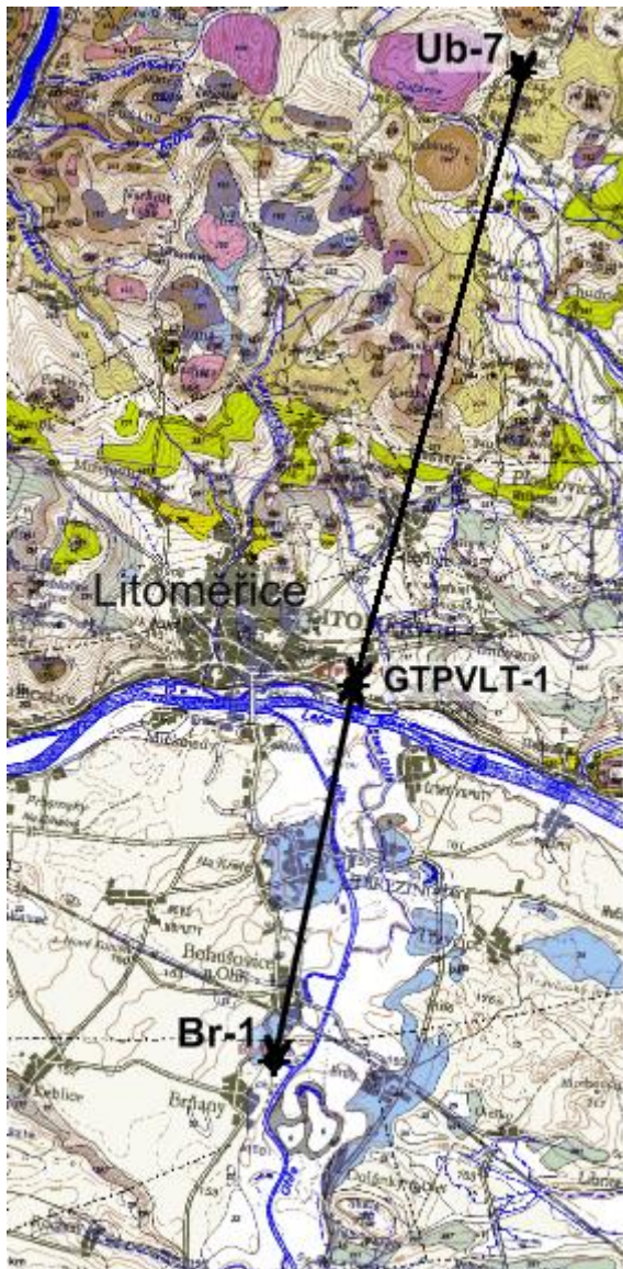
Figure 15 Boreholes Br-1, GTPV LT-1 and Úb-7 (from south to north) and the position of the geological section running through them in the section of a geological map 1:50 000 published by the Czech Geological Survey.
