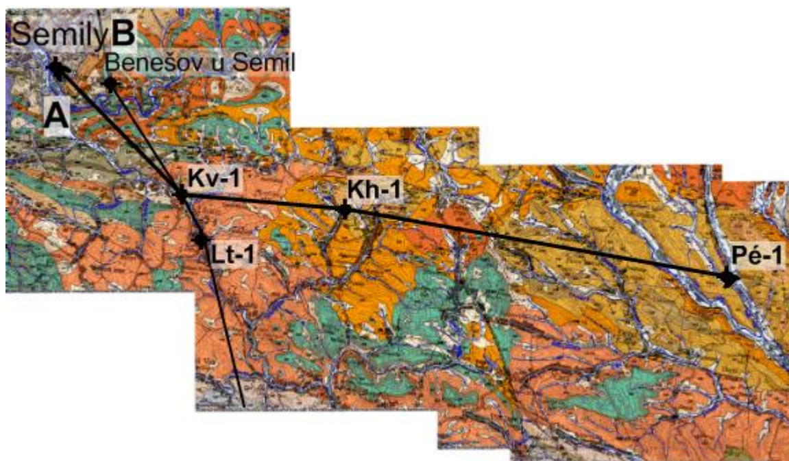
Figure 28 The town of Semily and boreholes Kv-1, Kh-1 and Pé-1 (from west to east) and the position of the geological sections A and B running through them in the section of a geological map 1:50 000 published by the Czech Geological Survey (composition from map sheets 03-41 Semily and 03-42 Trutnov).
