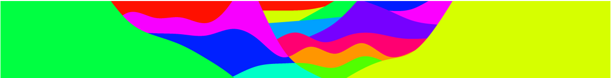
Figure 2: Blocks in model P1I. The colour of the block is determined by its index. The colour changes from green to red and blue. Block 1 is the leftmost green block.
