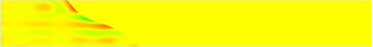
Figure 1: P-wave velocity perturbation between model P1-1-10% and the background model. Positive perturbations are red, negative perturbations are green. Zero perturbations are drawn yellow.
