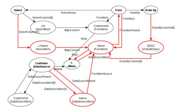
Figure 8.4: An example of affected elements of a query graph because of the DataSourceItem being removed.
