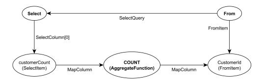
Figure 7.5: An example of a usage of an aggregate function in the SELECT clause.
