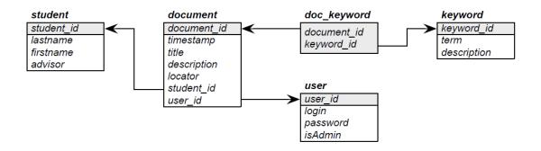
Figure 2.1: A sample of relational schema diagram
