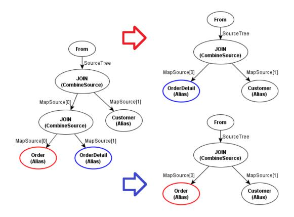
Figure 8.6: An example of a simple replacing of the parent of the removed alias with its sibling in the combination source tree.
