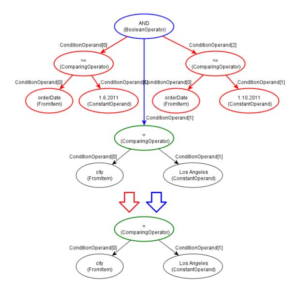
Figure 8.5: An example of reorganization of a condition because of removing of a FromItem vertex.
