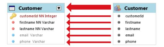
Figure 7.15: An example of a mapping between database model and query model.
