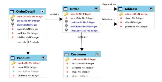
Figure 6.2: The example of PSM database model.
