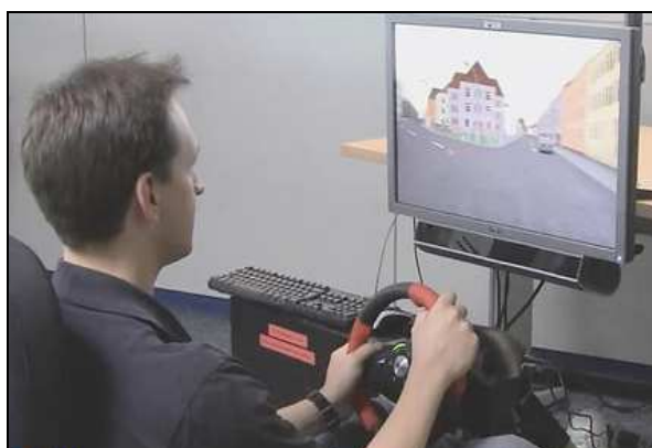
Obr. 10: Simulátor s remote eye-trackerem pod obrazovkou ( www.flickr.com )
