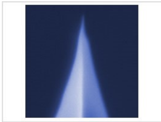
Fig. 5.14: Super sharp spike tip. The small spike is silicon tip processed for the first 200nm of the tip apex. Cantilever parameters: spring constant ( k ): 42N/m, resonant frequency ( f_0 ): 320 kHz. Tip parameters: tip radius ( R ): 2-5nm. Tip Height ( h ): 10 - 15 \mu m. Front Angle (FA): 25 \pm 2.5^\circ . Back Angle (BA): 15 \pm 2.5^\circ . Side Angle (SA): 22.5 \pm 2.5^\circ 55 .
