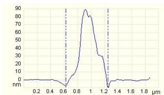
Fig. 9.20: Aggregates of the CFD2 nanoparticles. First row: topography of the sample, amplitude error and the height images. Second row: the cross section of the aggregate. Images were taken with MESP tip in TM.
