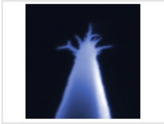
Fig. 5.15: Diamond-like carbon sharp tip (DLCS) by Veeco. Tip parameters are following: Tip Height (h): 15 - 20 \mu m. Front Angle (FA): 15 \pm 2^\circ . Back Angle (BA): 15 \pm 2^\circ . Side Angle (SA): 15 \pm 2^\circ . Tip Radius (R): 1-5nm. 55
