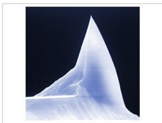
Fig. 5.12: Sharp silicon tip for tapping mode in detail. Tip parameters: Tip Height (h): 10 - 15 \mu m. Front Angle (FA): 25 \pm 2.5^\circ . Back Angle (BA): 15 \pm 2.5^\circ . Side Angle (SA): 22.5 \pm 2.5^\circ . Tip Radius (R): 8-10 nm. 55
