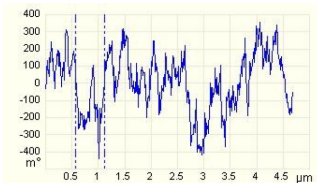
Fig. 10.18: The Co5 sample, magnetized in parallel orientation at 0.5 and 5 T, respectively. The magnetic phase images together with the cross-sections from the middle part of the image are illustrated. R_a is the value of the surface roughness.
